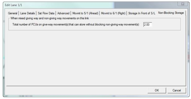
The only setting on the tab is the number of PCU at the front of the storage area which do not block Ahead traffic. In this case as shown above this is 2 PCU with the third Right Turn Storage PCU blocking the Ahead traffic.
