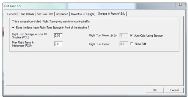
Lanes which include Right Turns that have Storage in front of the Stop Line require additional settings to model all the components of right turn capacity modelled by LinSig. These settings are contained on the 'Storage in Front of Stop Line' tab. They include:
