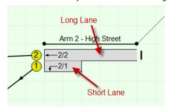
Where signalled Short Lanes are relatively long and are unlikely to empty during a typical green period they can generally be modelled as a Long Lane which can sometimes be useful in simplifying complex Lane arrangements.
