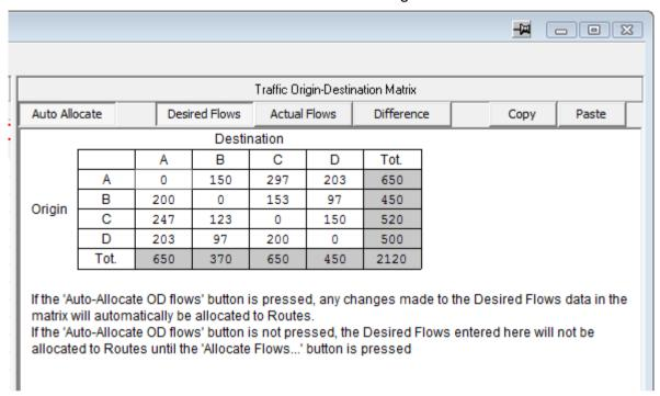
Traffic OD movements are specified using a single OD matrix for the entire network, however it is less meaningful to model pedestrians over such a large area therefore pedestrian OD matrices are specified using one OD matrix for each LinSig Junction. This makes the specification of pedestrian flows simpler.
