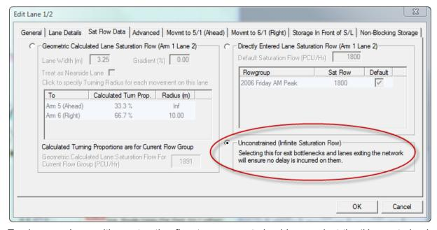
To change a Lane with a saturation flow to a unconstrained Lane select the 'Unconstrained (Infinite Saturation Flow)' option on the Saturation Flow Data tab.
