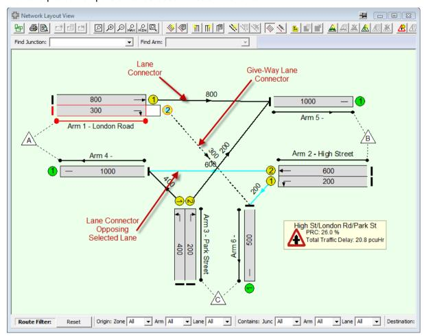
The diagram above shows Lane Connectors joining Lanes to other Lanes. Lane Connectors representing traffic movements which give way to other Lanes are shown dashed. If a give-way Lane or give-way Lane Connector is selected with the mouse its opposing Lane Connectors are shown highlighted.
