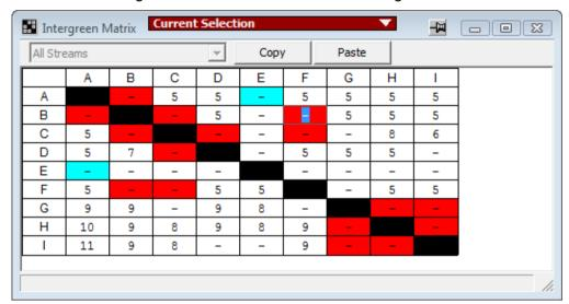
The Intergreens represent the safe clearance interval in seconds between the time a phase terminates and the time another phase starts. Advice on calculating Intergreens can be obtained in the DfT Advisory Leaflet TAL 1/06.
