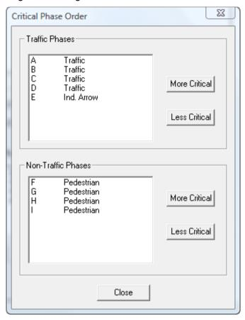
Phases are ordered in two separate lists: Traffic Phases and non-traffic Phases. Traffic Phases are always treated as higher priority than all non-traffic Phases.
