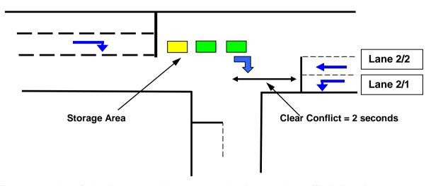
The mechanism of what happens with respect to the right turning traffic is directly dependant on the method of control. However, the parameters entered into LinSig are the same and LinSig uses them as appropriate depending on the method of control used.
