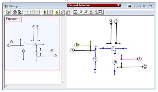
UK Stage View becomes Phase View. The Phase View shows the Phases defined for each Phase Stream in a Controller. The Phases are named alphanumerically and can have alternate Phases defined.
