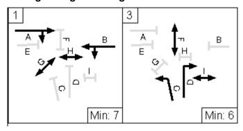
If the method of control is modified to provide an early cut off Stage (indicative arrow) as shown below, then right turners can turn in gaps during Stage 1, at full saturation flow during Stage 2 and will also receive a bonus for the number of vehicles stored in front of the stop line prior to Stage 2 starting.
