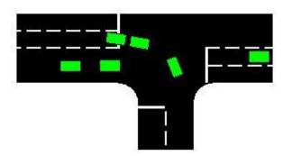
LinSig uses the give way model described above to model the capacity of the right turn during the period it is opposed by oncoming traffic. Common practice in the UK for many years has been to use Tanners formula to calculate the amount of traffic turning in gaps. This can be closely approximated in LinSig V3 by using 1440 for Intercept and 1.09 for slope in the give way model.
