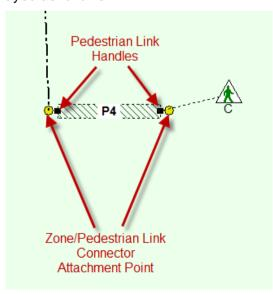
Pedestrian Links together with Pedestrian Link Connectors form a Pedestrian Network for each LinSig Junction. Pedestrian movements between junctions are not modelled. Due to issues such as pedestrian dispersion, crossing at places other than a controlled crossing and leaving the Network between Junctions modelling pedestrians over a wider area is complex and beyond what LinSig is intended to model.
