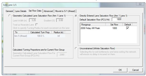
Lane Saturation Flows can be specified manually or can be calculated from a Lane's geometry using the formulae published in the TRRL report RR67. Saturation flows are always specified in Passenger Car Units (PCU) in LinSig.
