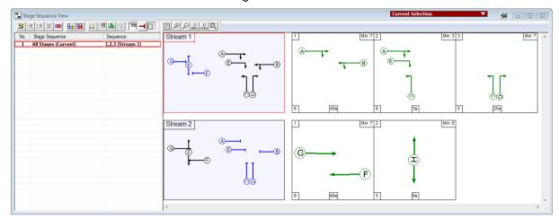
With Multiple Stage Streams are switched on LinSig requires a separate Stage Sequence to be defined for each Stage Stream. The Stage Sequence for each Stream is made up of Stages defined for that Stage Stream. Stages defined for a Stage Stream cannot be used in the Stage Sequences of different Stage Streams.
